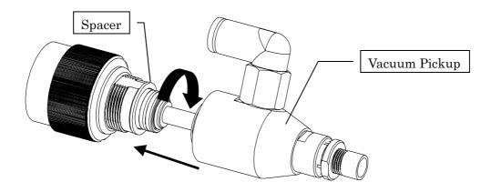
(3) Adjust the sleeve length according to the conditions of use.
