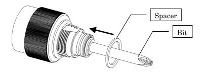
(2) Fix the Vacuum Pickup onto the screwdriver by turning it clockwise.
